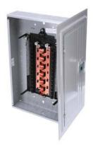
SIEMENS LOW VOLTAGE PL SERIES LOAD CENTER. MAIN LUG WITH 24 1-Inch Spaces ALLOWING MAX 30 CIRCUITS. 1-PHASE 3-WIRE SYSTEM RATED 120/240V(125A) 100KA INTERRUPT. SPECIAL FEATURES: COPPER BUS, INTERCHANGEABLE MAIN, SPLIT GROUND, GRAY TRIM, NEMA TYPE1 ENCLOSURE FOR INDOOR USE. REPLACED BY PN2448L1125C. AVAILABLE 4/1/2020
