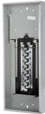
SIEMENS LOW VOLTAGE PL SERIES LOAD CENTER. MAIN LUG WITH 30 1-Inch Spaces ALLOWING MAX 40 CIRCUITS. 1-PHASE 3-WIRE SYSTEM RATED 120/240V(200A) 100KA INTERRUPT. SPECIAL FEATURES: ALUMINUM BUS, INTERCHANGEABLE MAIN, GRAY TRIM, NEMA TYPE1 ENCLOSURE FOR INDOOR USE. REPLACED BY PN3048L1200. AVAILABLE 4/1/2020
