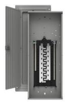
SIEMENS LOW VOLTAGE PL SERIES LOAD CENTER. MAIN LUG WITH 30 1-Inch Spaces ALLOWING MAX 40 CIRCUITS. 1-PHASE 3-WIRE SYSTEM RATED 120/240V(200A) 100KA INTERRUPT. SPECIAL FEATURES: ALUMINUM BUS, INTERCHANGEABLE MAIN, SPLIT GROUND, GRAY TRIM, NEMA TYPE1 ENCLOSURE FOR INDOOR USE. REPLACED BY PN3048L1200. AVAILABLE 4/1/2020
