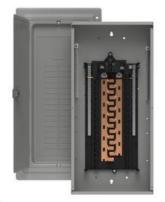
SIEMENS LOW VOLTAGE PL SERIES LOAD CENTER. FACTORY INSTALLED MAIN BREAKER WITH 30 1-INCH SPACES ALLOWING MAX 42 CIRCUITS. 1-PHASE 3-WIRE SYSTEM RATED 120/240V (125A) 22KA INTERRUPT. SPECIAL FEATURES: COPPER BUS, INTERCHANGEABLE MAIN, CUSTOM BUILD, GRAY TRIM, NEMA TYPE1 ENCLOSURE FOR INDOOR USE. REPLACED BY PN3030B1125C. AVAILABLE 4/1/2020
