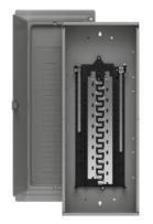
SIEMENS LOW VOLTAGE PL SERIES LOAD CENTER. MAIN LUG WITH 40 1-Inch Spaces ALLOWING MAX 40 CIRCUITS. 1-PHASE 3-WIRE SYSTEM RATED 120/240V(200A) 100KA INTERRUPT. SPECIAL FEATURES: ALUMINUM BUS, INTERCHANGEABLE MAIN, SPLIT GROUND, GRAY TRIM, NEMA TYPE1 ENCLOSURE FOR INDOOR USE. REPLACED BY PN4040L1200. AVAILABLE 4/1/2020
