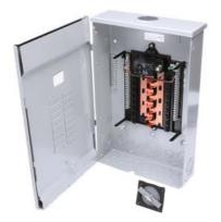
SIEMENS LOW VOLTAGE PL SERIES LOAD CENTER. FACTORY INSTALLED MAIN BREAKER WITH 12 1-INCH SPACES ALLOWING MAX 24 CIRCUITS. 1-PHASE 3-WIRE SYSTEM RATED 120/240V (100A) 22KA INTERRUPT. SPECIAL FEATURES: COPPER BUS, INTERCHANGEABLE MAIN, GRAY TRIM, NEMA TYPE3R ENCLOSURE FOR OUTDOOR USE. REPLACED BY PNW1224B1100C. AVAILABLE 4/1/2020
