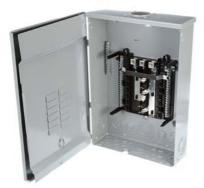
SIEMENS LOW VOLTAGE PL SERIES LOAD CENTER. MAIN LUG WITH 12 1-INCH SPACES ALLOWING MAX 24 CIRCUITS. 3-PHASE 4-WIRE SYSTEM RATED 120/240V OR 120/208V (125A) 100KA INTERRUPT. SPECIAL FEATURES: COPPER BUS, INTERCHANGEABLE MAIN, GRAY TRIM, NEMA TYPE3R ENCLOSURE FOR OUTDOOR USE.
