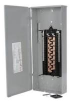
SIEMENS LOW VOLTAGE PL SERIES LOAD CENTER. MAIN LUG WITH 30 1-Inch Spaces ALLOWING MAX 40 CIRCUITS. 1-PHASE 3-WIRE SYSTEM RATED 120/240V(125A) 100KA INTERRUPT. SPECIAL FEATURES: COPPER BUS, INTERCHANGEABLE MAIN, GRAY TRIM, NEMA TYPE3R ENCLOSURE FOR OUTDOOR USE. REPLACED BY PNW3048L1125C. AVAILABLE 4/1/2020
