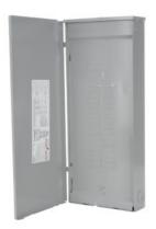
SIEMENS LOW VOLTAGE PL SERIES LOAD CENTER. MAIN LUG WITH 30 1-Inch Spaces ALLOWING MAX 40 CIRCUITS. 1-PHASE 3-WIRE SYSTEM RATED 120/240V(200A) 100KA INTERRUPT. SPECIAL FEATURES: COPPER BUS, INTERCHANGEABLE MAIN, GRAY TRIM, NEMA TYPE3R ENCLOSURE FOR OUTDOOR USE. REPLACED BY PNW3048L1200C. AVAILABLE 4/1/2020
