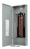
SIEMENS LOW VOLTAGE PL SERIES LOAD CENTER. MAIN LUG WITH 40 1-Inch Spaces ALLOWING MAX 40 CIRCUITS. 1-PHASE 3-WIRE SYSTEM RATED 120/240V(200A) 100KA INTERRUPT. SPECIAL FEATURES: COPPER BUS, INTERCHANGEABLE MAIN, GRAY TRIM, NEMA TYPE3R ENCLOSURE FOR OUTDOOR USE. REPLACED BY PNW4040L1200C. AVAILABLE 4/1/2020
