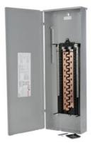
SIEMENS LOW VOLTAGE PL SERIES LOAD CENTER. MAIN LUG WITH 42 1-Inch Spaces ALLOWING MAX 60 CIRCUITS. 1-PHASE 3-WIRE SYSTEM RATED 120/240V(225A) 100KA INTERRUPT. SPECIAL FEATURES: COPPER BUS, INTERCHANGEABLE MAIN, GRAY TRIM, NEMA TYPE3R ENCLOSURE FOR OUTDOOR USE. REPLACED BY PNW4264L1225C. AVAILABLE 4/1/2020
