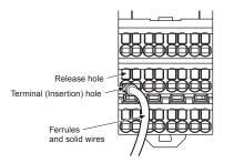
• If a wire is difficult to connect because it is too thin, use a flat-blade screwdriver in the same way as when connecting stranded wire.
