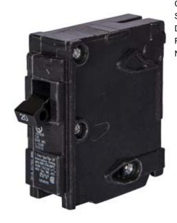
Siemens Low Voltage Residential Circuit Breakers Miniature Thermal Mag Circuit Breakers - Special App are Circuit Protection Load Center Mains, Feeders, and Miniature Circuit Breakers. Type: QP Special Features: High-Intensity Discharge Application: Electrical Distribution Standard: UL 489 Voltage Rating: 120V Amperage Rating: 20A Trip Range: Thermal Magnetic Interrupt Rating: 10 AIC Number Of Poles: 1P
