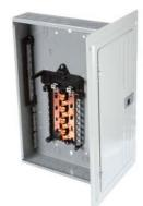
SIEMENS LOW VOLTAGE RISER LOAD CENTER. MAIN LUG WITH 16 1-INCH SPACES ALLOWING MAX 32 CIRCUITS. 1-PHASE 3-WIRE SYSTEM RATED 120/240V (125A) 100KA INTERRUPT. SPECIAL FEATURES: COPPER BUS, INTERCHANGEABLE MAIN, GRAY TRIM.
