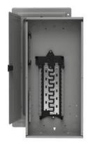
SIEMENS LOW VOLTAGE RISER LOAD CENTER. MAIN LUG WITH 24 1-INCH SPACES ALLOWING MAX 24 CIRCUITS. 1-PHASE 3-WIRE SYSTEM RATED 120/240V (125A) 100KA INTERRUPT. SPECIAL FEATURES: ALUMINUM BUS, INTERCHANGEABLE MAIN, GRAY TRIM.
