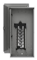
SIEMENS LOW VOLTAGE RISER LOAD CENTER. MAIN LUG WITH 24 1-INCH SPACES ALLOWING MAX 42 CIRCUITS. 1-PHASE 3-WIRE SYSTEM RATED 120/240V (125A) 100KA INTERRUPT. SPECIAL FEATURES: COPPER BUS, INTERCHANGEABLE MAIN, GRAY TRIM.
