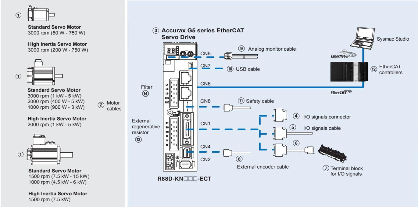
**Note:** The symbols ①②③④⑤... show the recommended sequence to select the components in Accurax G5 servo system
