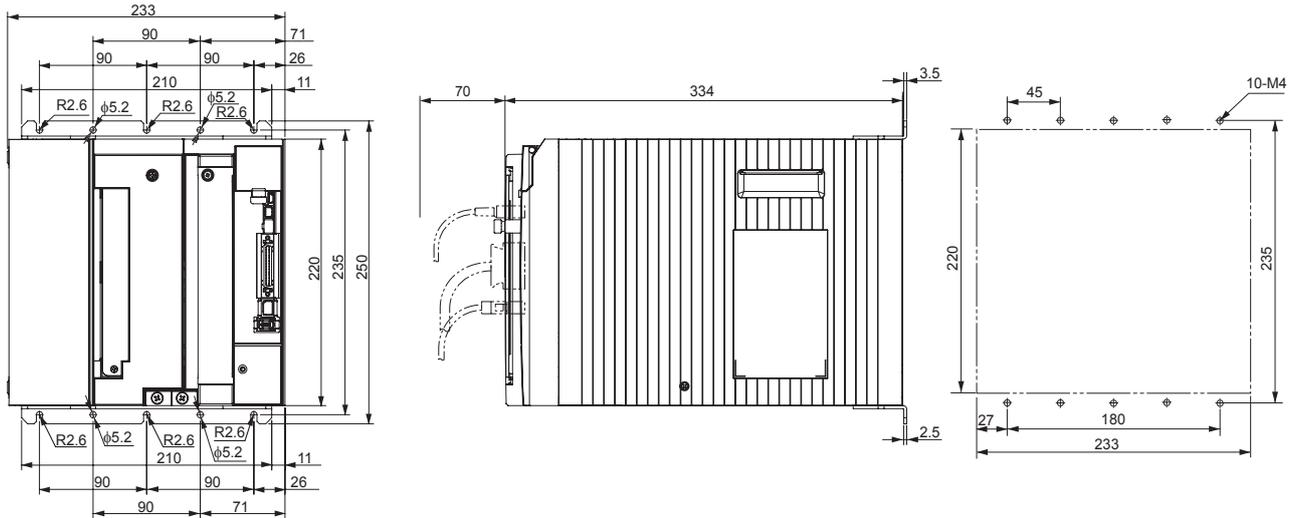
R88D-KT150F, R88D-KN150H-ECT (400 V, 15 kW)
