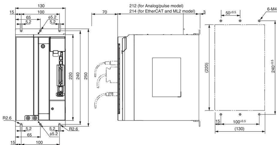
R88D-KT75F, R88D-KN75H-ECT (400 V, 7.5 kW)
