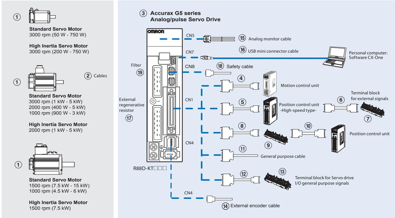
Note: The symbols ①②③④⑤... show the recommended sequence to select the components in Accurax G5 servo system
