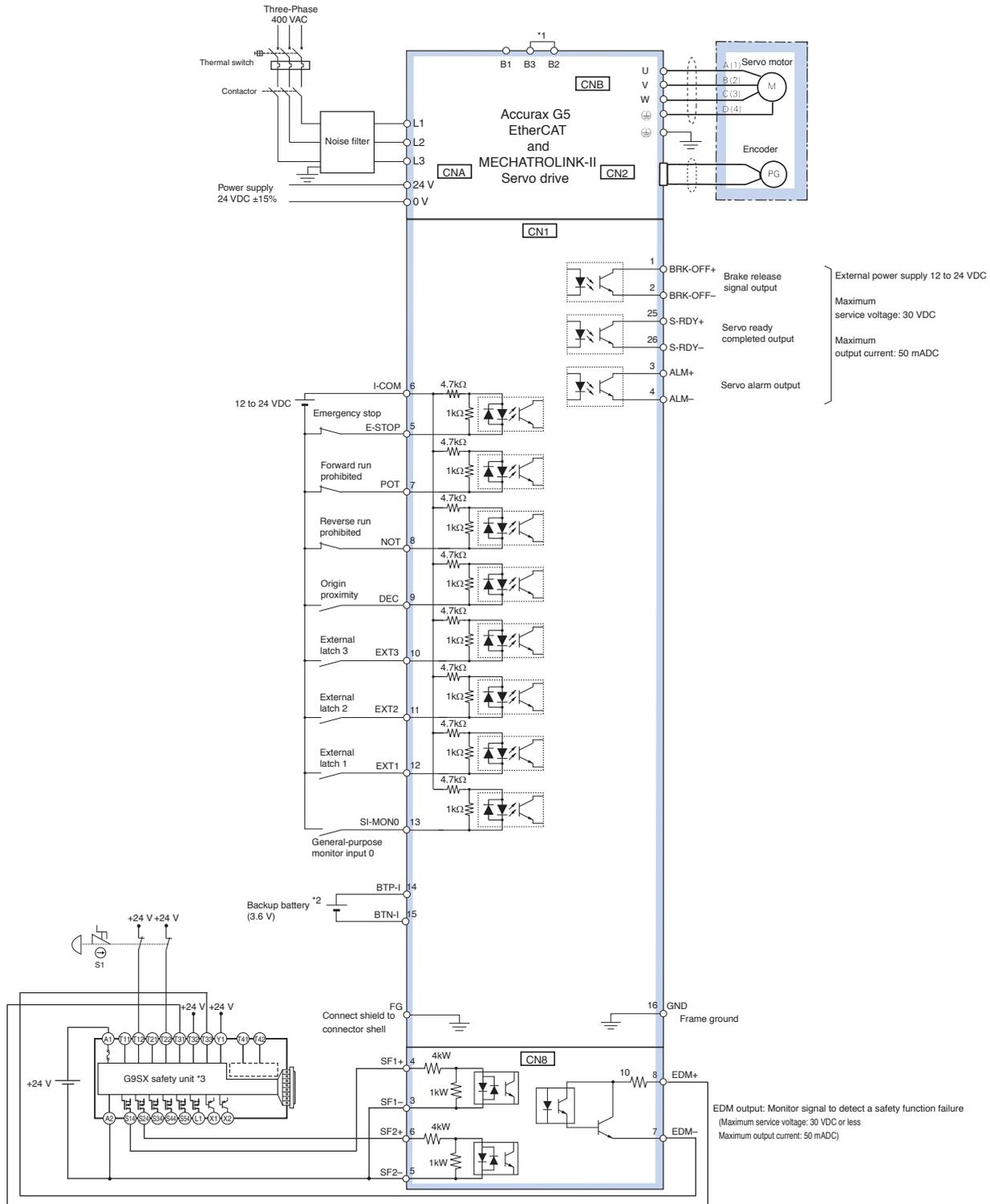
\*1 Normally B2 and B3 are short-circuited. If the internal regenerative resistor is insufficient, remove the wire between B2 and B3 and connect an external regenerative resistor between B1 and B2.
