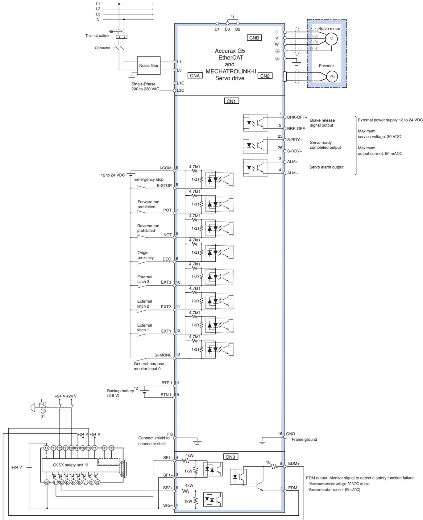
\*1 For servo drives from 750 W, B2 and B3 are short-circuited. If the internal regenerative resistor is insufficient, remove the wire between B2 and B3 and connect an external regenerative resistor between B1 and B2.
