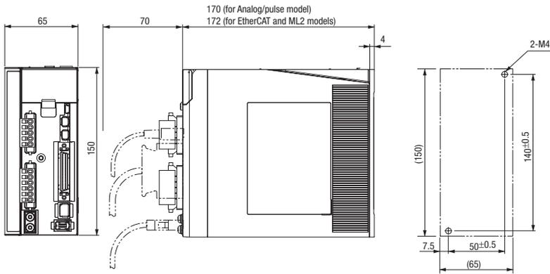
R88D-KT10/15H, R88D-KN10/15H-□ (230 V, 1 to 1.5 kW)
