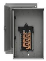
SIEMENS LOW VOLTAGE MURRAY RISER LOAD CENTER. MAIN LUG WITH 16 1-INCH SPACES ALLOWING MAX 32 CIRCUITS. 1-PHASE 3-WIRE SYSTEM RATED 120/240V (125A) 100KA INTERRUPT. SPECIAL FEATURES: COPPER BUS, INTERCHANGEABLE MAIN, GRAY TRIM.
