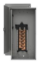
SIEMENS LOW VOLTAGE MURRAY RISER LOAD CENTER. MAIN LUG WITH 24 1-INCH SPACES ALLOWING MAX 24 CIRCUITS. 1-PHASE 3-WIRE SYSTEM RATED 120/240V (125A) 100KA INTERRUPT. SPECIAL FEATURES: COPPER BUS, INTERCHANGEABLE MAIN, GRAY TRIM.
