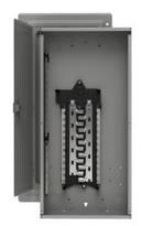
SIEMENS LOW VOLTAGE MURRAY RISER LOAD CENTER. MAIN LUG WITH 24 1-INCH SPACES ALLOWING MAX 42 CIRCUITS. 1-PHASE 3-WIRE SYSTEM RATED 120/240V (125A) 100KA INTERRUPT. SPECIAL FEATURES: COPPER BUS, INTERCHANGEABLE MAIN, GRAY TRIM.
