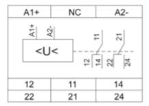
A1+,A2-: Voltage to be monitored 11-14,12: 1st C/O contact of output relay 21-24,22: 2nd C/O contact of output relay
