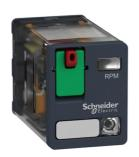
plug-in relay, Harmony electromechanical relays, 15A, 2CO, with LED, lockable test button, 230V AC
