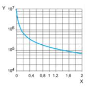
X Switching capacity (kVA) Y Durability (Number of operating cycles) Reduction coefficient for inductive AC load (depending on power factor cos φ)
