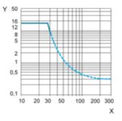
X Voltage DCY Current DCNote : These are typical curves, actual durability depends on load, environment, duty cycle, etc.
