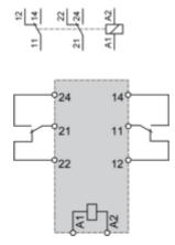
**NOTE:** For DC input, A1 have to be +, otherwise it would short circuit from protection module
