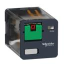
Harmony, Universal plug-in relay, 10 A, 2 CO, with lockable test button, flat (faston) terminals, 24 V AC
