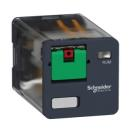
Harmony, Universal plug-in relay, 10 A, 2 CO, with lockable test button, flat (faston) terminals, 48 V AC
