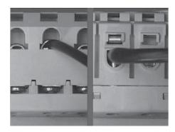
Conductors may only be inserted into open terminals, preventing mis-wiring and potential problems.
