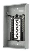
SIEMENS LOW VOLTAGE ES SERIES LOAD CENTER. MAIN LUG WITH 24 1-Inch Spaces ALLOWING MAX 40 CIRCUITS. 1-PHASE 3-WIRE SYSTEM RATED 120/240V(125A) 100KA INTERRUPT. SPECIAL FEATURES: ALUMINUM BUS, FACTORY INSTALLED GROUND BAR, GRAY TRIM, NEMA TYPE1 ENCLOSURE FOR INDOOR USE. REPLACED BY SN2448L1125. AVAILABLE 4/1/2020
