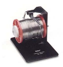
Keeps the working area tidy and reduces solder wastage. The solder wire is led from the solder dispenser through a guiding tube. The SD1000 can be positioned for the soldering job in such a way that the hands of the operator are free for the soldering iron and the component to be soldered.
