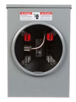
Siemens Low Voltage Talon Meter Sockets Residential - Talon Meter Sockets UAT1 Steel are Residential Enclosures Single-Family Metering. Type: UAT1 Special Features: NO BYPASS Application: RESIDENTIAL Standard: UL Voltage Rating: 300V Amperage Rating: 135A Phase: 1 OR 3 PHASE Size: 4.800X8.600X13.200 Cable Entry: UG Terminal: 5 TERMINALS Mounting: SURFACE MOUNTING Operating Temperature: AVERAGE AMBIENT Enclosure: STEFI
