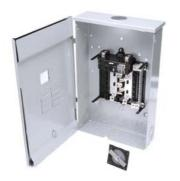
SIEMENS LOW VOLTAGE ES SERIES LOAD CENTER. FACTORY INSTALLED MAIN BREAKER WITH 8 1-INCH SPACES ALLOWING MAX 16 CIRCUITS. 1-PHASE 3-WIRE SYSTEM RATED 120/240V (200A) 22KA INTERRUPT. SPECIAL FEATURES: ALUMINUM BUS, FEED-THRU LUGS, GRAY TRIM, NEMA TYPE3R ENCLOSURE FOR OUTDOOR USE. REPLACED BY SNW0816B1200T. AVAILABLE 4/1/2020
