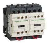
NEMA Contactor, TeSys N, reversing, Size 00, 9A, 2HP at 460VAC, 3 pole, 3 phase, 24VDC coil, open
