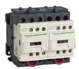
NEMA Contactor, TeSys N, reversing, Size 1, 27A, 10HP at 460VAC, 3 pole, 3 phase, 24VDC coil, open
