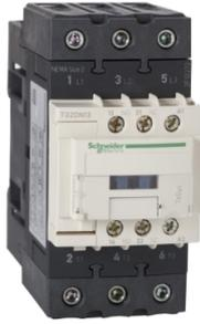
Contactor, TeSys N Contactors, nonreversing, 3P, 3phase, 45A, 25HP at 460VAC, NEMA size 2, 208VAC 50/60Hz coil, open
