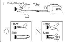
**2.** After inserting, grasp the handle tightly and insert the end of the tubing to the stroke end.
