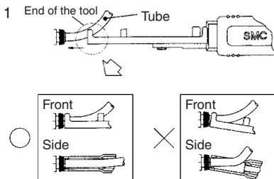
2. After inserting, grasp the handle tightly and insert the end of the tubing to the stroke end.
