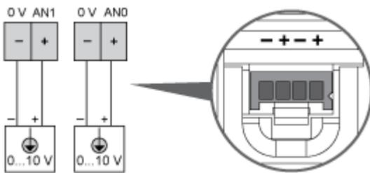
The (-) poles are connected internally.
