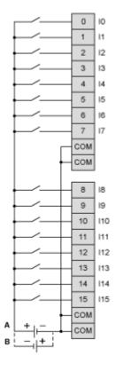
The 4 COM terminals are connected internally
