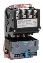
Non-reversing motor starter, Size 00, Three phase full voltage, Solid-state overload relay, OLRelay amp range 0.75-3.4a, 380 440/440 480V 50/60HZ coil, Non-combination type, Enclosure type (open), No enclosure
