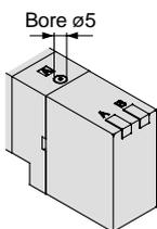
Push down the manual override button with a small screwdriver until it stops.
