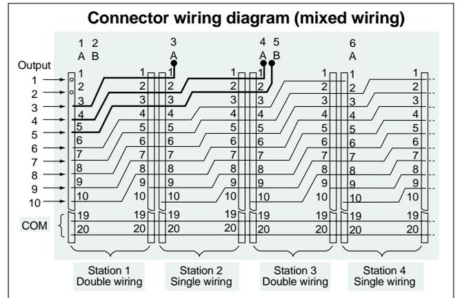
(Refer to the connector wiring diagram)
