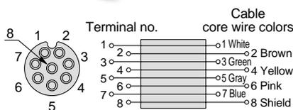
Socket connector pin arrangement
