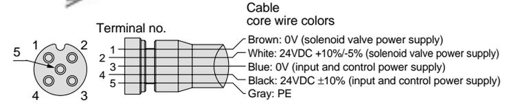
Socket connector pin arrangement
