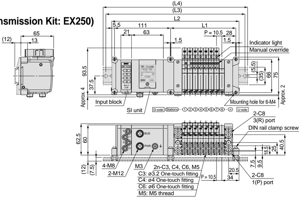
Formulas: L1 = 10.5n + 45, L2 = 10.5n + 167.5 (for 1 input block. For each additional input block, add 21mm.) n: Stations (maximum 24 stations)
