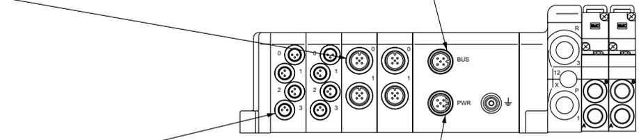
● **Communication connector (PROFIBUS-DP): M12, 5 pins (plug)**
