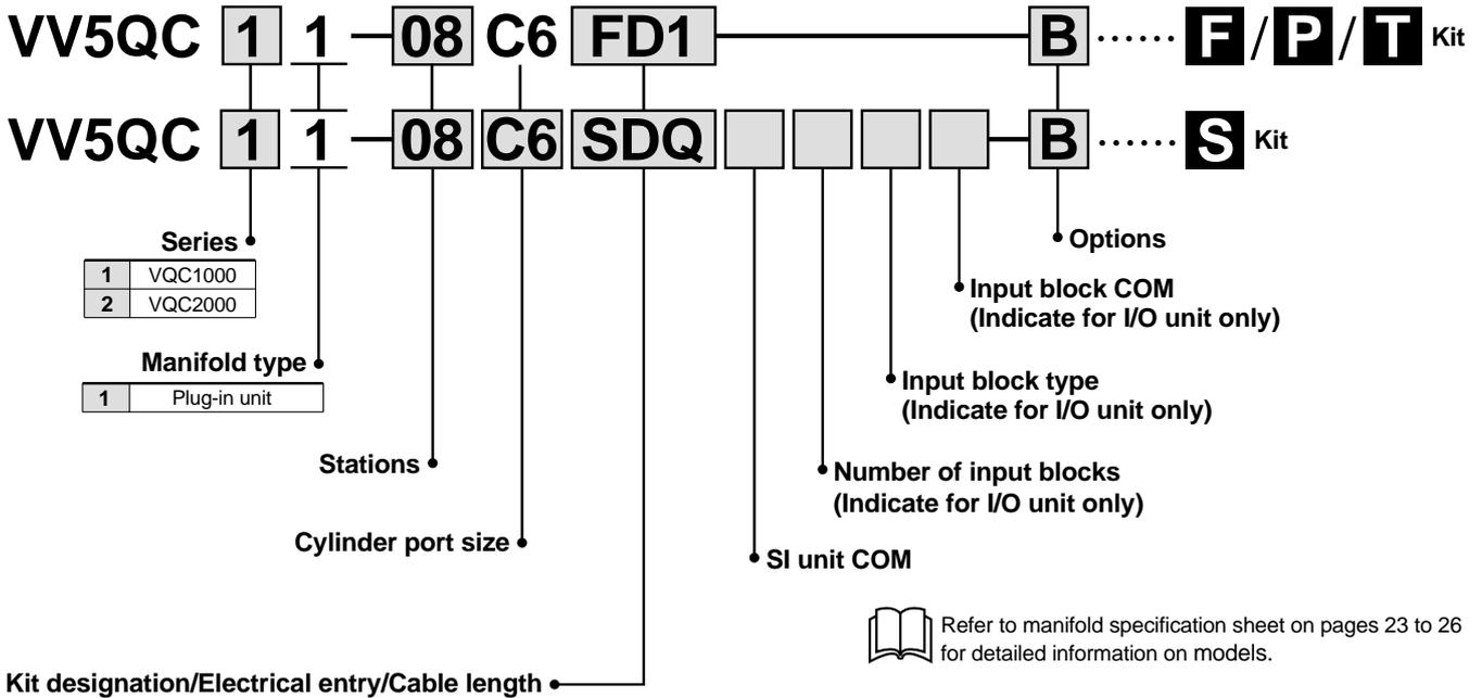
**S** Kit (Decentralized wiring type serial transmission kit)
