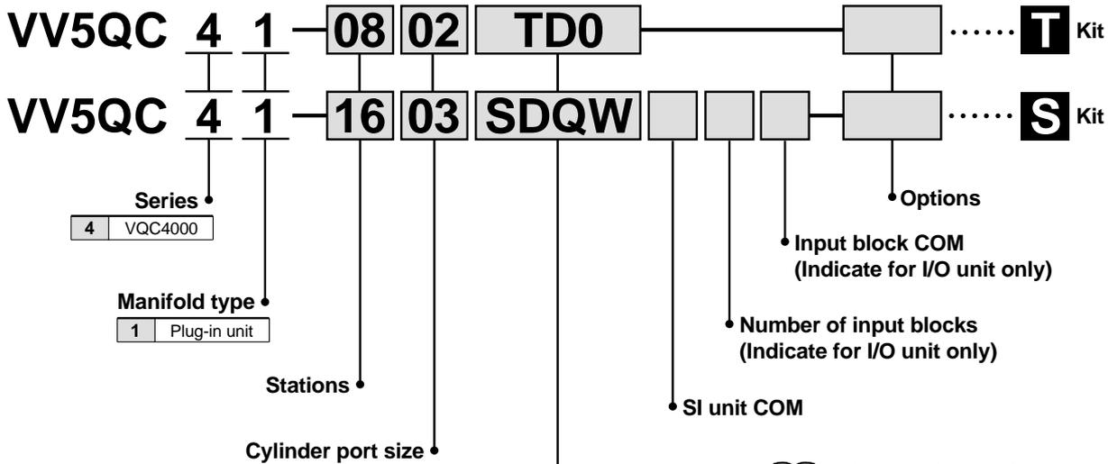
Refer to manifold specification sheet on pages 27 and 28 for detailed information on models.
