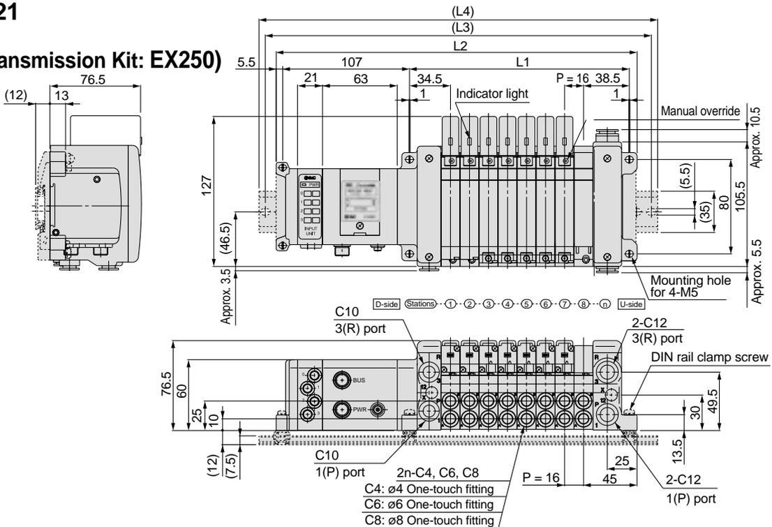
Formulas: L1 = 16n + 57, L2 = 16n + 176 (for 1 input block. For each additional input block, add 21mm.) n: Stations (maximum 24 stations)
