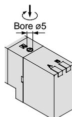
Push down the manual override button with a small flat head screwdriver until it stops, and turn it clockwise 90° to lock it. Turn it counterclockwise to release it.
