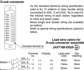
used is for 12 stations or less, double wiring (connected to SOL. A and SOL. B) is used for the internal wiring of each station regardless Mixed single and double wiring are available
