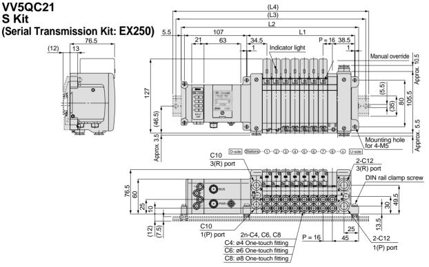
Formulas: L1 = 16n + 57, L2 = 16n + 176 (for 1 input block. For each additional input block, add 21mm.) n: Stations (maximum 24 stations)
