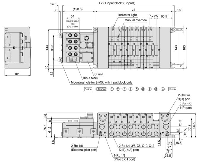
Formulas: L1 = 25n + 106, L2 = 25n + 241 (for 1 input block. For each additional input block, add 54mm.) n: Stations (maximum 16 stations)
