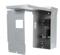
Siemens Energy Management Residential Specialty Load centers: small circuit (2-10). Sub Brand: Load Centers Type: 1: Application: Residential: Voltage Rating: 120/240V Amperage rating: 100A Phase: 1PH Load regulation: 100 A Wiring configuration: 3w Bus Rating: 100 A Interrupt rating: 22000AIC. EQ LC 2S 4C MB 100A 3R
