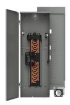
SIEMENS LOW VOLTAGE GENERATOR READY LOADCENTER. FACTORY INSTALLED MAIN BREAKER WITH 30 1-INCH SPACES ALLOWING MAX 42 CIRCUITS. 1-PHASE 3-WIRE SYSTEM RATED 120/240V (200A) 22KA INTERRUPT. SPECIAL FEATURES: TIN PLATED COPPER BUS, (GENERAC), NEMA TYPE3R ENCLOSURE FOR OUTDOOR USE.
