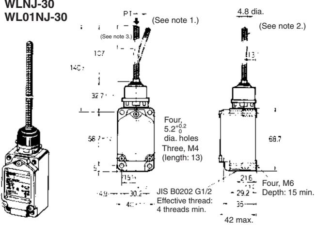
**Note: 1.** The coil spring may be operated from any direction except the axial direction (↓).
