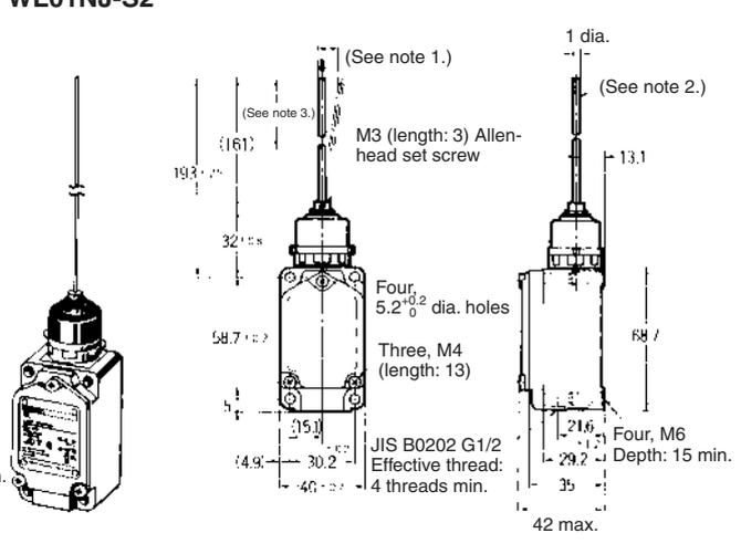
**Note: 1.** The coil spring may be operated from any direction except the axial direction (↓).
