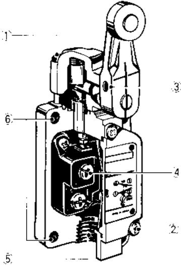
In particular, when changing the direction of the Head, make sure that all screws are tightened again to the correct torque. Do not allow foreign objects to fall into the Switch.
