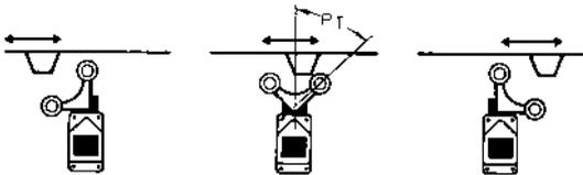
NC terminal: ON    NO terminal: ON    NO terminal: ON
