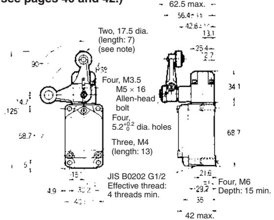
Note: Plastic roller. This illustration shows the external dimensions of the WLCA32-41. (Models WLCA32-041 to -044 and WL01CA32-041 to -044 have stainless steel rollers.)
