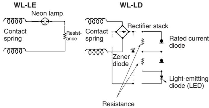
■ Wiring Specifications of Sensor I/O Connector Models
