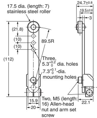
**Note:** Can be installed on the rear side.
