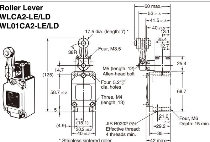
Note: Unless otherwise indicated, a tolerance of ±0.4 mm applies to all dimensions.
