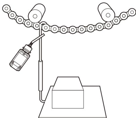
**Pallet Detection in Arc Welding Lines**
