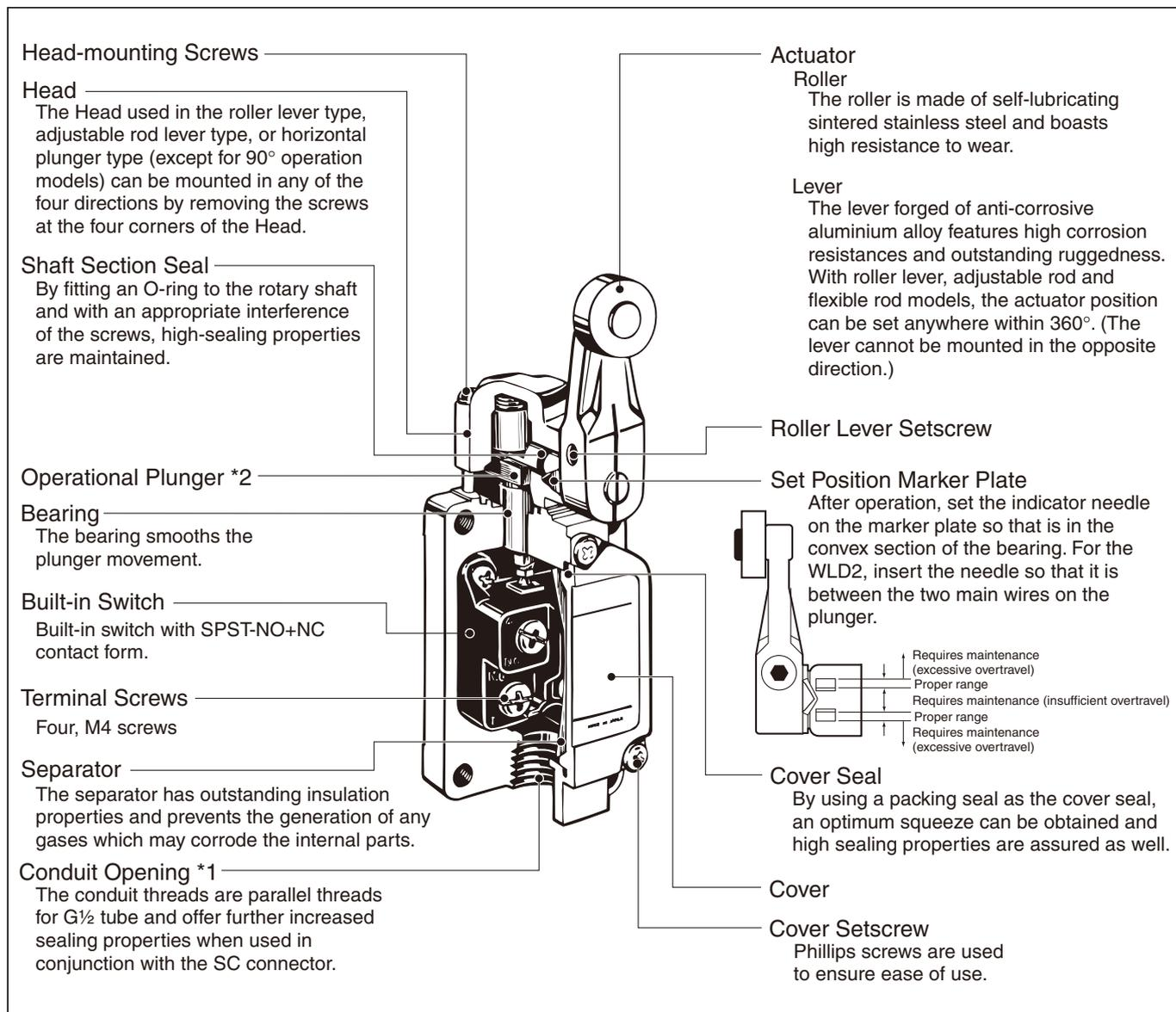
\*1. The display for conduit threads has changed from PF½ to G½, according to revisions of JIS B 0202. This is only a change in the display, so the thread size and pitch have not changed. (Conduit threads Pg 13.5 and ½-14NPT are also available.)
