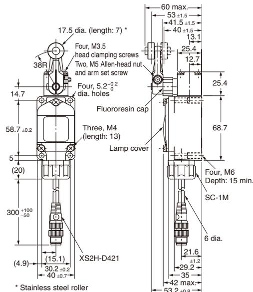
Sealed Top-roller Plunger (Screw Terminals)
