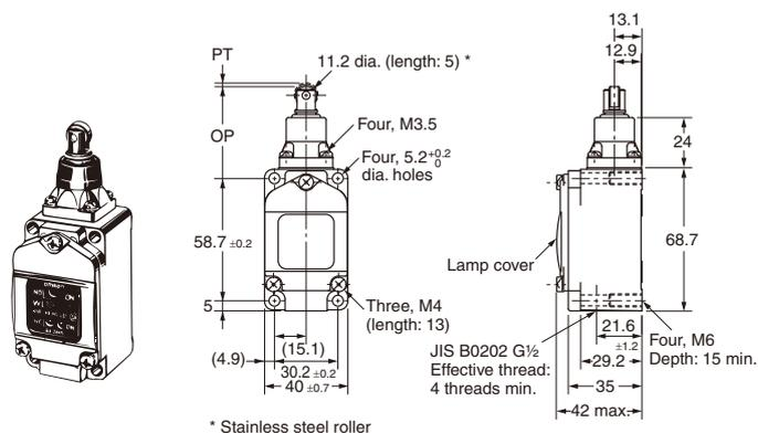
Sealed Top-roller Plunger (Pre-wired connectors)
