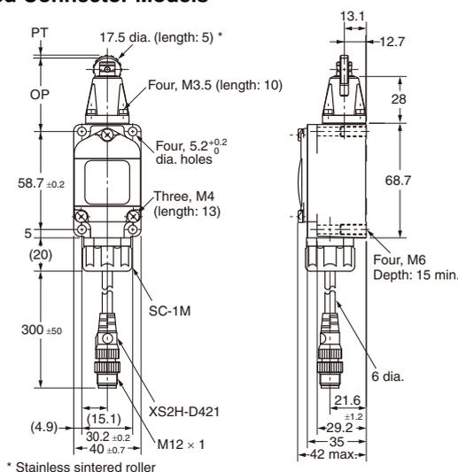
Note: 1. Unless otherwise indicated, a tolerance of ±0.4 mm applies to all dimensions.
