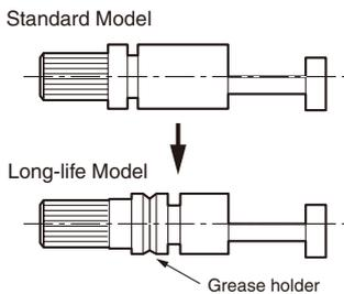
Smooth movement is achieved using olefin grease. (Standard models use molybdenum disulfide grease.)
