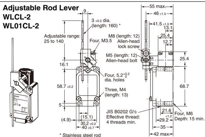
Note: 1. With the side-installation models, 90° operation on one side is possible by simply changing the direction of the cam.
