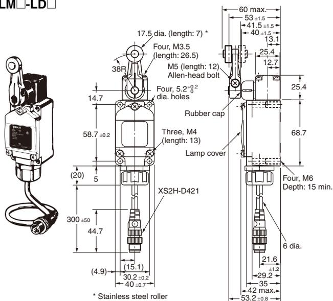
Note: Unless otherwise indicated, a tolerance of ±0.4 mm applies to all dimensions.
