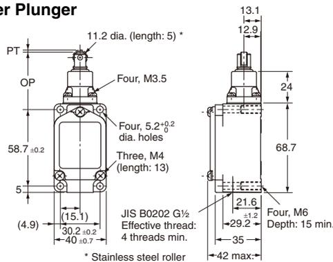
Note: Unless otherwise indicated, a tolerance of ±0.4 mm applies to all dimensions.
