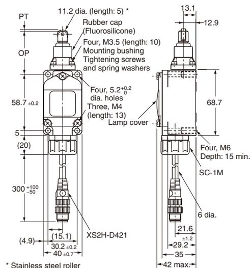
Note: Unless otherwise indicated, a tolerance of ±0.4 mm applies to all dimensions.
