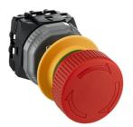
Emergency stop push button, Harmony XB5, plastic, red, mushroom 40mm, 22mm, trigger latching turn to release, monitoring contact, 1NO 2NC
