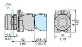
**e:** clamping thickness: 1 to 6 mm / 0.04 to 0.24 in. **(1)** Additional row of contacts or double contact.
