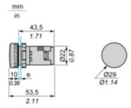
e: clamping thickness: 1 mm to 6 mm / 0.03 in. to 0.24 in.
