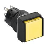
Illuminated monolithic push button, Harmony XB6E, square yellow flush, 16mm, spring return 12VDC, 1CO
