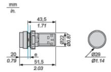
e Support panel thickness: 1 to 6 mm/0.4 to 0.24 in. (metal), 2 to 6 mm/0.8 to 0.24 in. (plastic).
